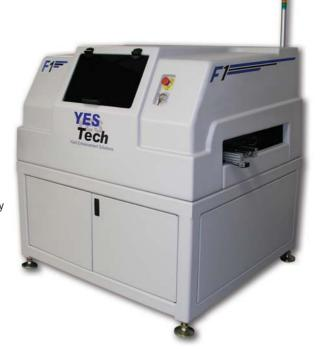
Programming the F1-Series is fast and intuitive. Operators typically take less than 30 minutes to create a complete inspection program including solder inspection. The F1-Series utilizes a standard package librate to simplify training and insure program portability across manufacturing lines.
